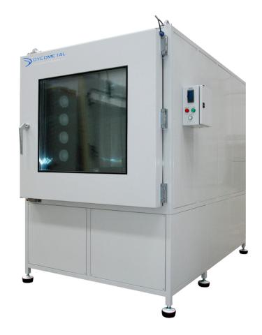
The Thermal Tests Chambers are used to make processes of accelerated thermal stress with controlled cold and heat tests
