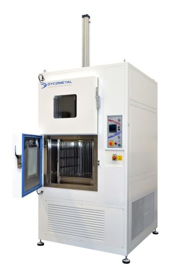
Very useful for performing Tests about the damage of the structure of a sample because of sudden changes of temperature. If these Thermal Shock or Impact Tests are made in a cyclical way, they can cause dilatations, deformations or even a breaking of the structure of the sample, electric mistakes in its connection or many affections in its physical and chemical properties.
