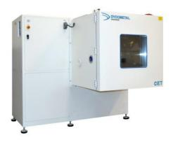
The development of these chambers is to perform a test of vibration and climate in parallel.
