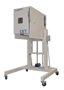
Tests in universal testing machines enable you to check the strength of the materials. In some tests, its require the conditioning of the samples, so its necessary to introduce between the columns of the universal test machine a chamber which can control the temperature parameters.
