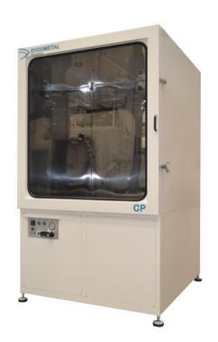
Within tests for evaluation of tightness of samples, other tests to be performed on electronics components are the powder Chambers, for determination of the degree of protection against solid agents.
