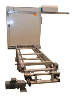
Airbag modules have to be conditioning under different temperatures and after this, they explode for the quality control. This explosion can be done inside or outside of the chamber, so this point affect to the construction of the chamber.
