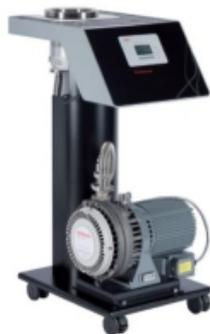
Leybold vacuum equipment (Pump + Turbo station) up to x10-6
