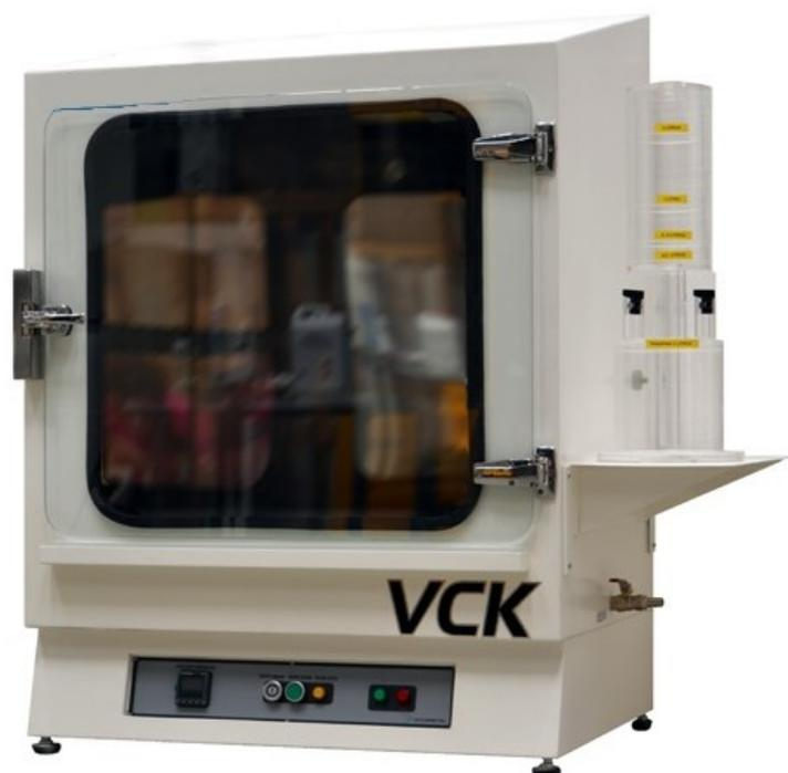
The Kesternich Corrosion Test has been designed to simulate industrial or urban atmospheres by means of the creation of an artificial atmosphere, by adding Sulphurous Anhydrid to the air, with or without Carbon Dioxide.
